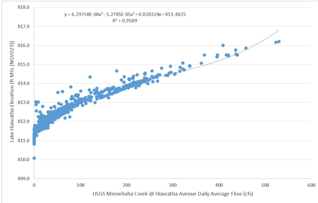
**Figure 10 Regression between USGS Gage on Minnehaha Creek and Lake Hiawatha Elevations**
