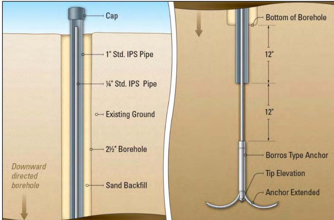
Figure 4 Borros-Type Settlement Point for Manual Monitoring (Geokon-1950)
