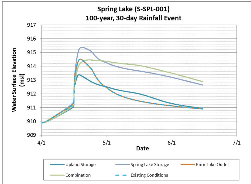
**Figure 4-12 Comparison of 100-year, 30-day Spring Lake water elevations resulting from flood damage reduction scenario simulations**
