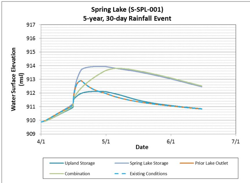
**Figure 4-4 Comparison of 5-year, 30-day Spring Lake water elevations resulting from flood damage reduction scenario simulations**
