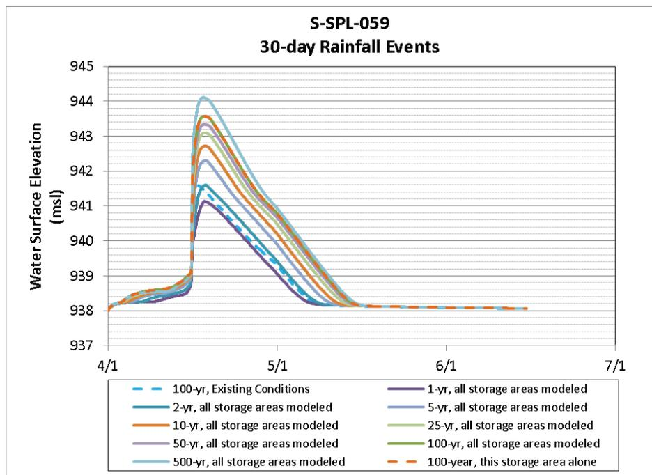
**Figure 3-6 Existing and Proposed Conditions Elevations for Potential Storage Area S-SPL-059**
