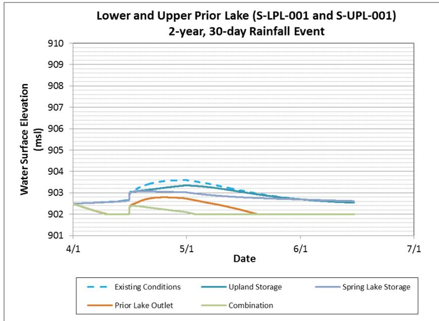
**Figure 4-3 Comparison of 2-year, 30-day Prior Lake water elevations resulting from flood damage reduction scenario simulations**
