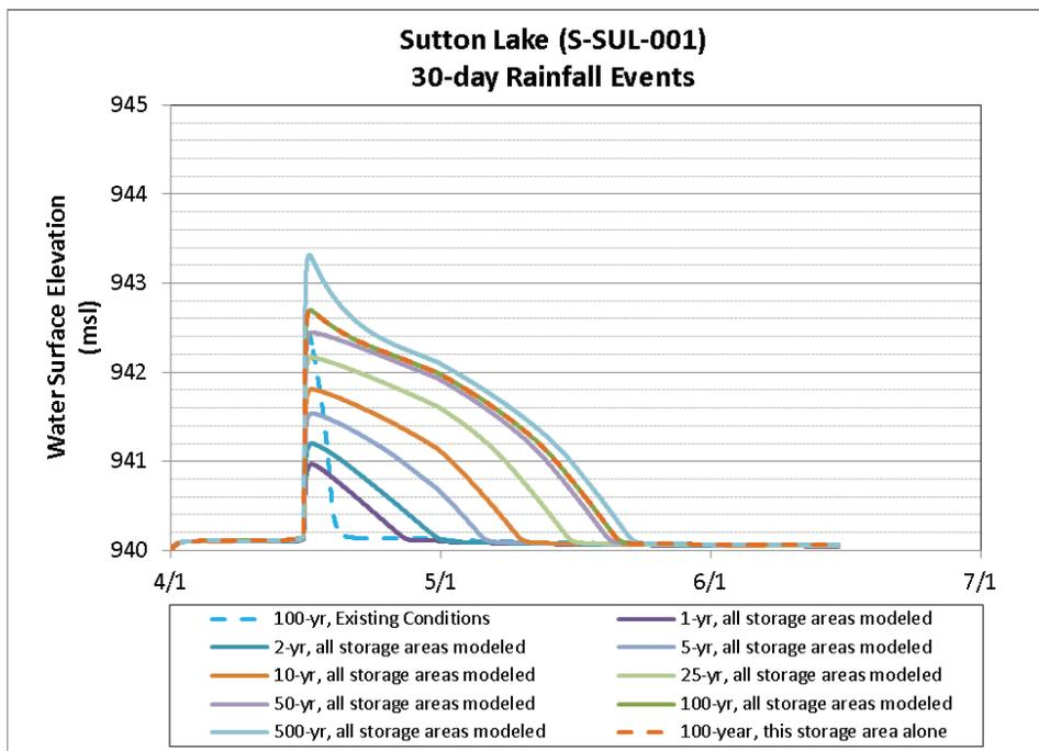
**Figure 3-10 Existing and Proposed Conditions Elevations for Potential Storage Area S-SUL-001**
