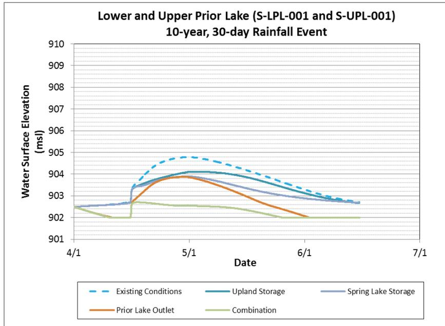
**Figure 4-7 Comparison of 10-year, 30-day Prior Lake water elevations resulting from flood damage reduction scenario simulations**
