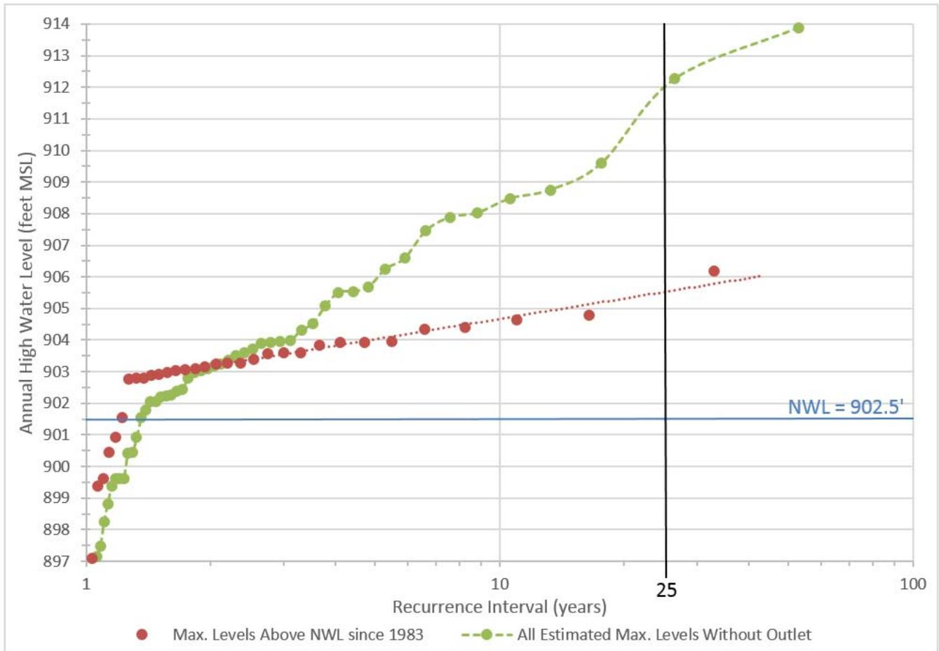
**Figure 2-6** Prior Lake Annual High Water Frequency Analyses With and Without Lake Outlet
