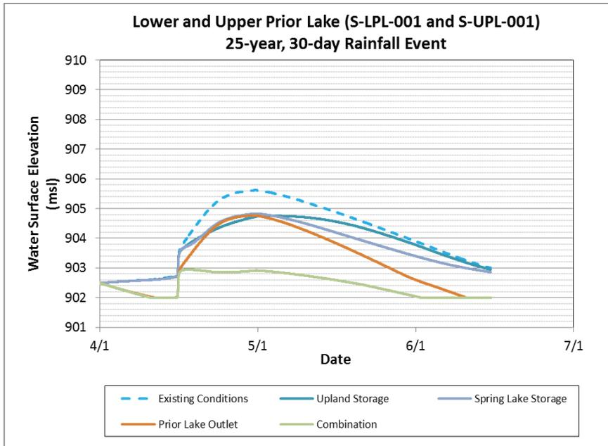
**Figure 4-9 Comparison of 25-year, 30-day Prior Lake water elevations resulting from flood damage reduction scenario simulations**
