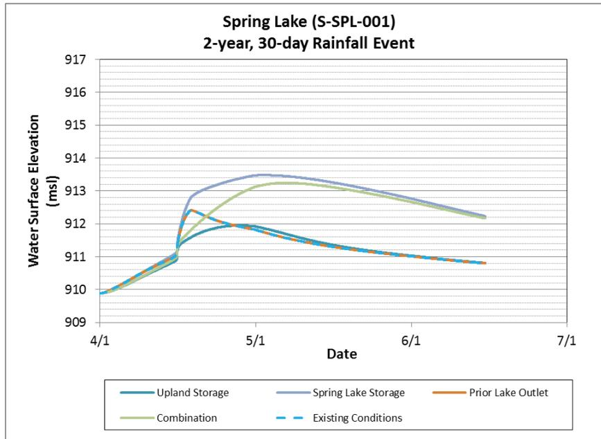
**Figure 4-2 Comparison of 2-year, 30-day Spring Lake water elevations resulting from flood damage reduction scenario simulations**
