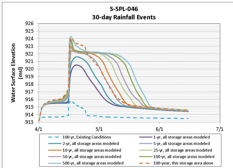
**Figure 3-4 Existing and Proposed Conditions Elevations for Potential Storage Area S-SPL-046**
