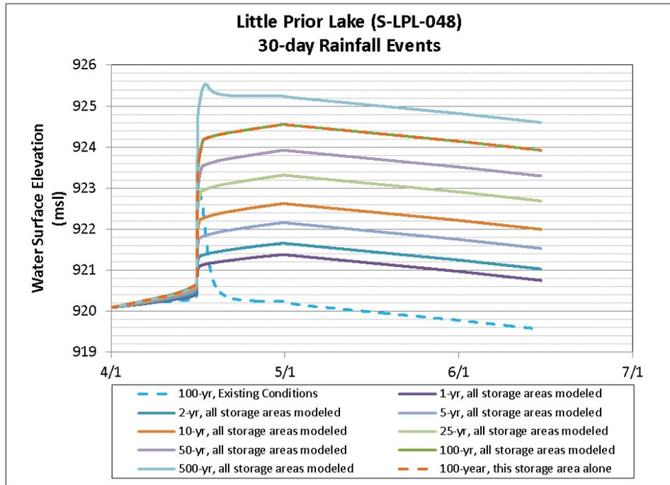
**Figure 3-3 Existing and Proposed Conditions Elevations for Potential Storage Area S-LPL-048**
