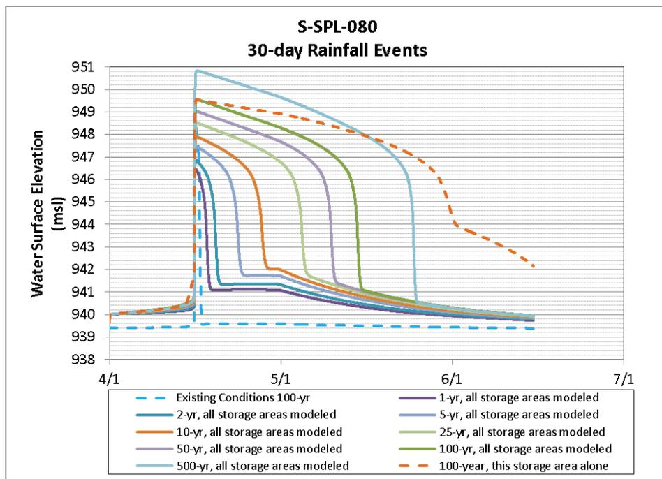
**Figure 3-8 Existing and Proposed Conditions Elevations for Potential Storage Area S-SPL-080**
