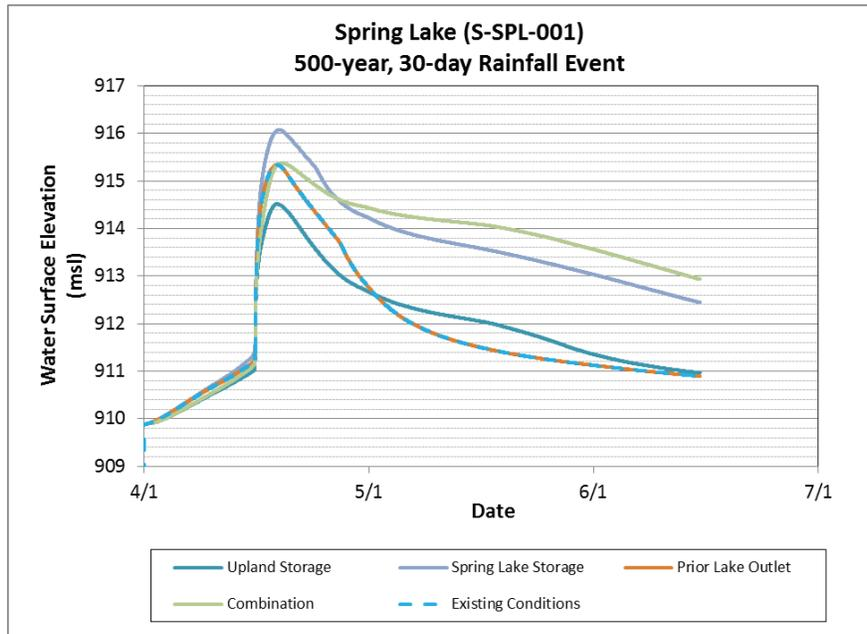
**Figure 4-14 Comparison of 500-year, 30-day Spring Lake water elevations resulting from flood damage reduction scenario simulations**
