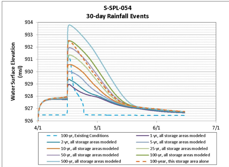
**Figure 3-5 Existing and Proposed Conditions Elevations for Potential Storage Area S-SPL-054**
