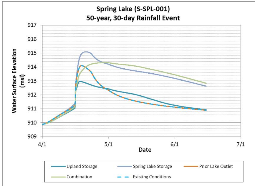
**Figure 4-10 Comparison of 50-year, 30-day Spring Lake water elevations resulting from flood damage reduction scenario simulations**
