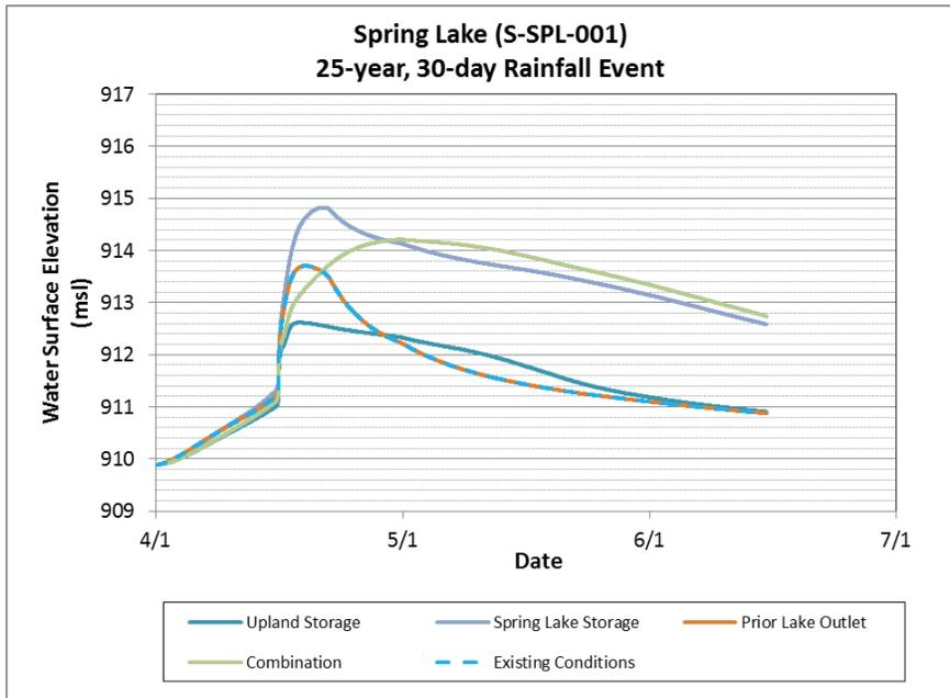
**Figure 4-8 Comparison of 25-year, 30-day Spring Lake water elevations resulting from flood damage reduction scenario simulations**
