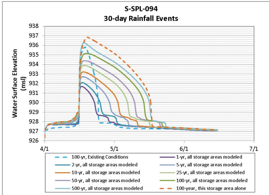
**Figure 3-9 Existing and Proposed Conditions Elevations for Potential Storage Area S-SPL-094**
