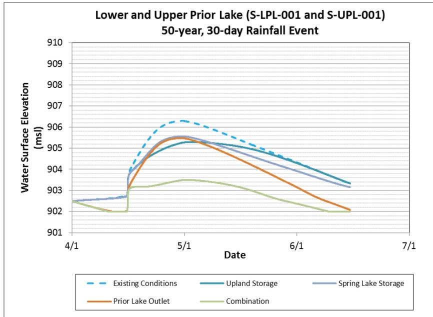
**Figure 4-11 Comparison of 50-year, 30-day Prior Lake water elevations resulting from flood damage reduction scenario simulations**
