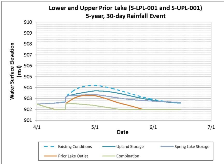
**Figure 4-5 Comparison of 5-year, 30-day Prior Lake water elevations resulting from flood damage reduction scenario simulations**
