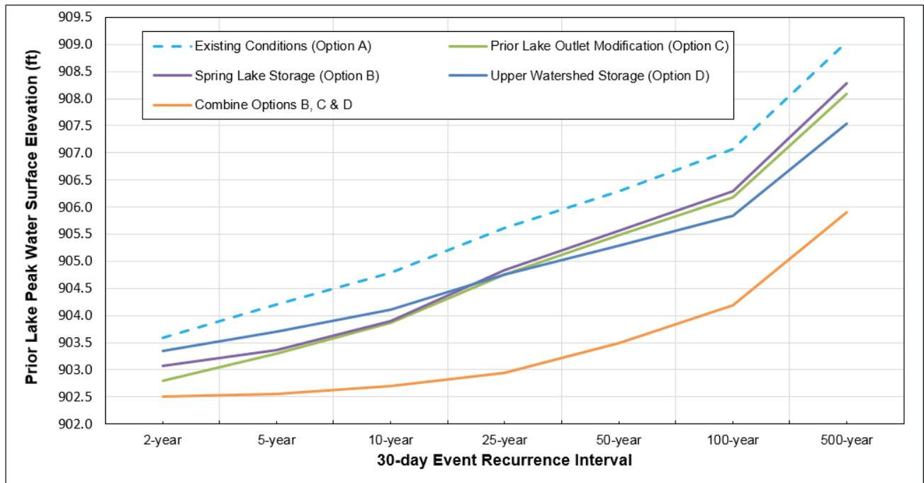
**Figure 7-2 Simulated Prior Lake flood levels for existing conditions and flood mitigation options**
