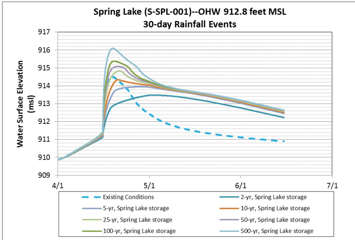
Figure 7-1 Existing and proposed conditions elevations for Spring Lake with modified outlet
