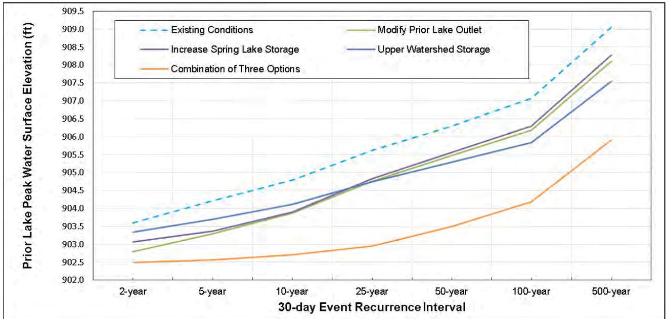
**Figure 4-1 Comparison of simulated Prior Lake Peak Elevations for existing conditions and flood damage reduction measures**
