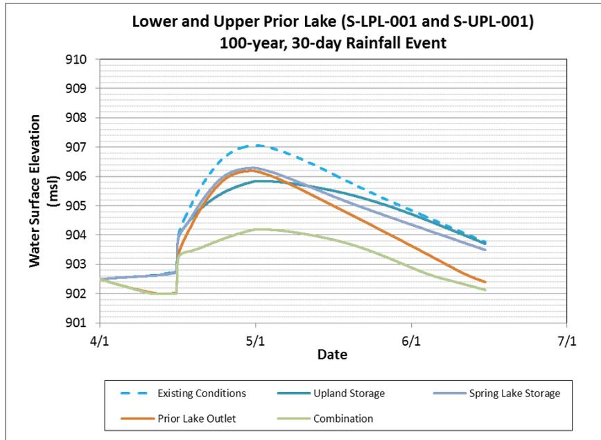
**Figure 4-13 Comparison of 100-year, 30-day Prior Lake water elevations resulting from flood damage reduction scenario simulations**
