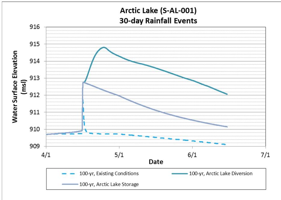
Figure 3-13 Arctic Lake 100-year, 30-day water surface elevations for existing conditions and for proposed conditions with the two Arctic Lake alternatives
