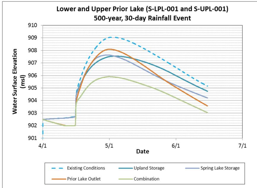
**Figure 4-15 Comparison of 500-year, 30-day Prior Lake water elevations resulting from flood damage reduction scenario simulations**
