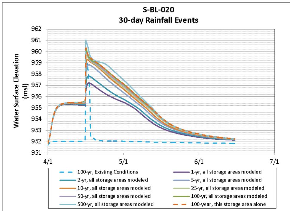
Figure 3-2 Existing and Proposed Conditions Elevations for Potential Storage Area S-BL-020
