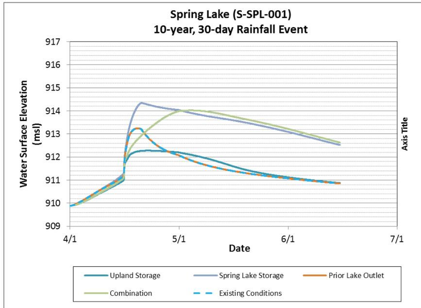
**Figure 4-6 Comparison of 10-year, 30-day Spring Lake water elevations resulting from flood damage reduction scenario simulations**
